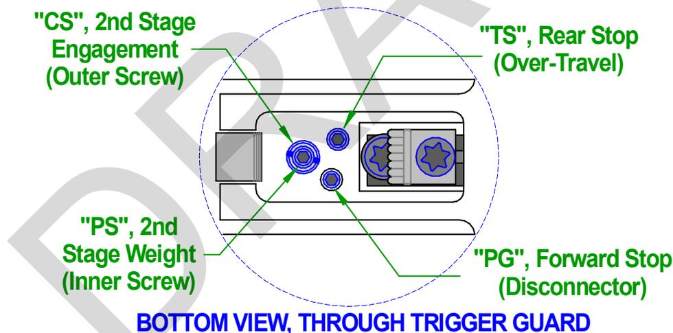
All of the set screws require a 1.5mm hex key. Screw "CS" requires a flat bladed screw driver. The factory supplied tool pouch has the appropriate hex key, but Pardini does not supply a suitable screwdriver for screw "CS". The blade needs to be about 4.5 - 5 mm wide and ~ 1 mm thick.
