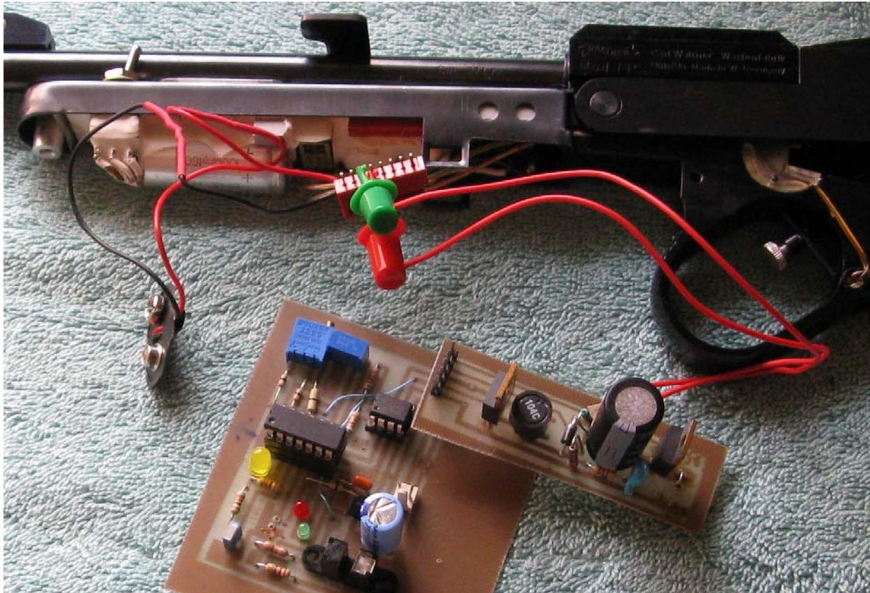
*In this first test board the 14 pin PIC and other logic components are on the big board. The small board is the SMPS high voltage converter. Large, TO-220 FETS are seen on the small board. The slot device on the big board is an optointerruptor to simulate the trigger.*
