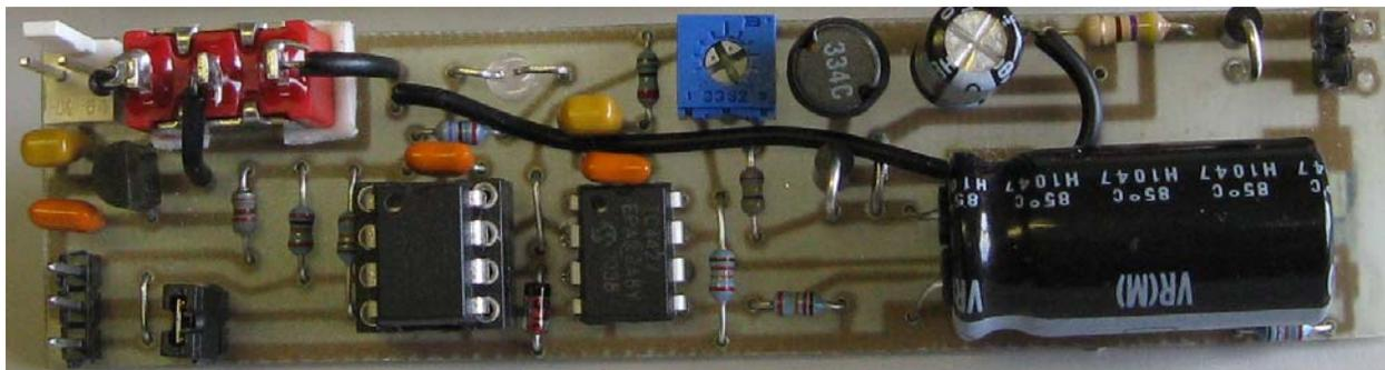
*In the photo see simple “snap apart” headers for P1, P2, and P3, while Figure 2 displays “KK” type headers. In the photo the battery connector, P4, is a KK connector. The PIC is installed in a socket while U2, the TC4427A, is soldered to the board. Q1 and Q2 are mounted on the back of the board, as is the jumper below R1. Note how few parts there are.*
