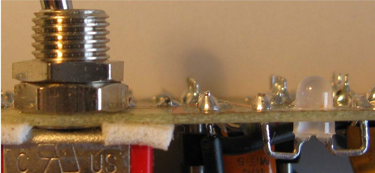
*This photo shows details of the diode, D4, installation and power switch. Note the compressed double stick tape that secures the power switch to the board. Note how close the switch mounting nuts are to the edge of the board. Filing the edge of the nuts may be necessary.*
