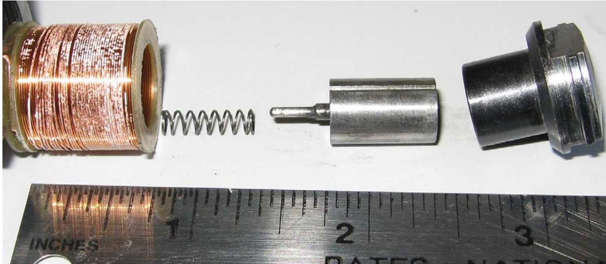
*Note the simplicity of the firing pin mechanism. The coil is four layers deep.*
