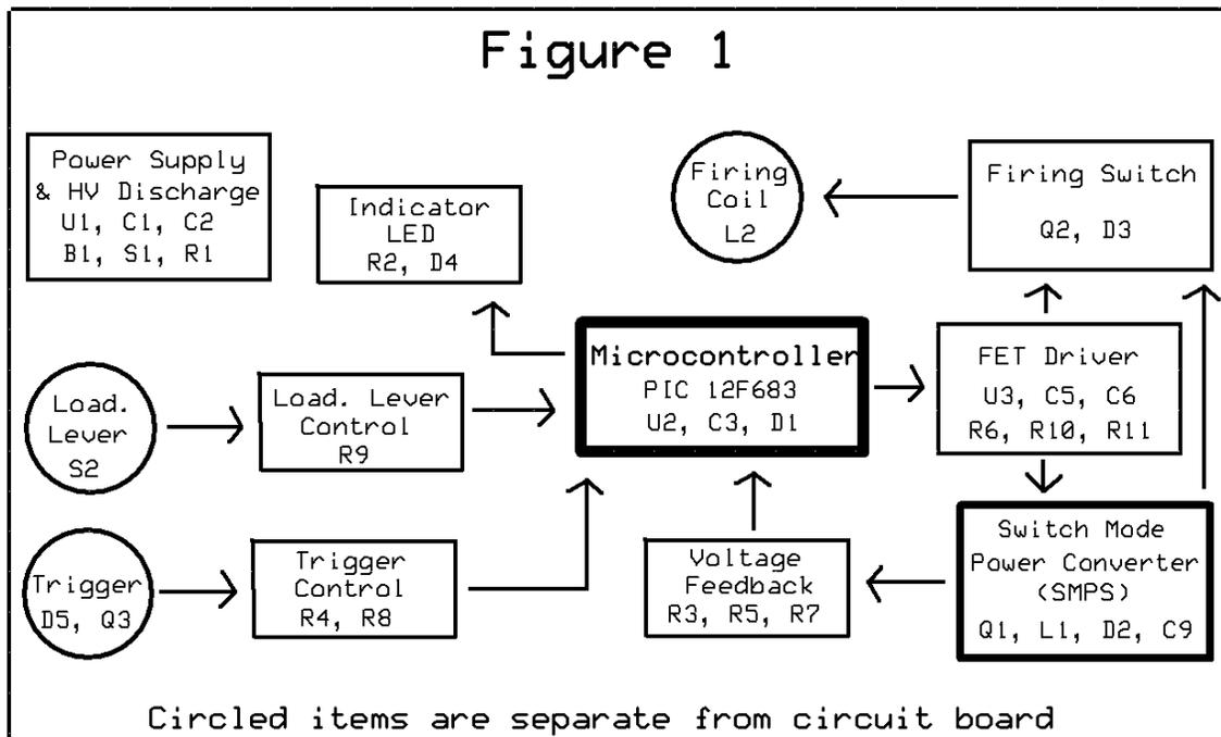
The Loading Lever tells the PIC whether the gun breech is open or closed. The loading lever switch is mounted beside the circuit board inside the pistol.
