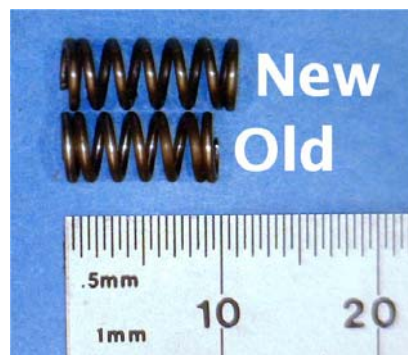
Figure 2: Old and new valve springs
